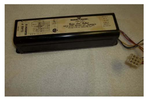
This is a rapid start ballast. Rapid starts are often pre-wired with a plug-in connector as seen here.
