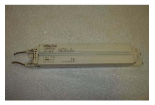
Here is an example of a "choke start ballast. The 2 wires at the left, attach to screws.
