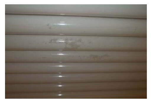
Before a thorough bed cleaning, you can see the dust that has accumulated on the inside of the canopy acrylic. This is what the customer sees while tanning. This dust is absorbing the UV.
