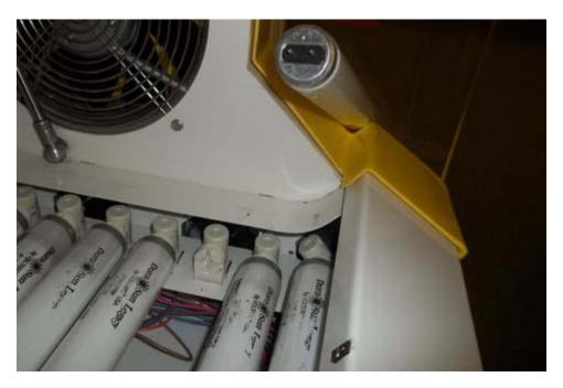
This is an example of a bi-pin with starter. The lamp at the top of the picture leaning against the frame of the bed is the bi-pin end. You will also notice in this picture that this tanning unit has closely packed reflector lamps and does not use an aluminum reflector behind the lamp. At the top of each lamp is where the starter is located and attached to the holder.
