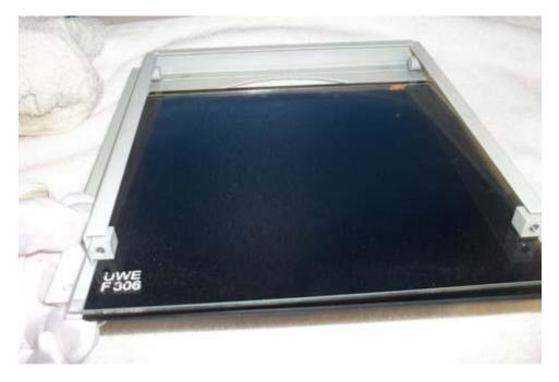
Here is a "cassette" of filter glass. A cassette is a holder used in high-pressure units that holds both blue and clear filter glass.
