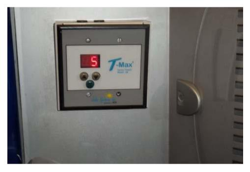
This is an example of an in-room timer. This timer can be mounted on the wall or the bed frame, in this picture the timer is mounted on the bed frame. The client presses the blue button to start the bed.
