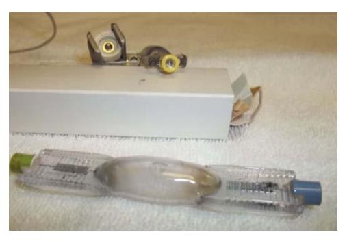
The top of this example shows the snap-in lamp holder to the left and the end view of the lamp to it's right. A full view of a snap in lamp is shown on the bottom of the picture. Snap-in lamps are usually mounted horizontally. Copyright 1994 - 2025 SunFocus Page 79
