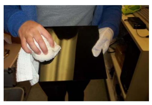
This person has removed the blue glass from the cassette above and is cleaning it with rubbing alcohol. Notice that he has a glove on one hand and a lint-free towel in the other. This is to ensure he does not touch the glass with his bare hands.
