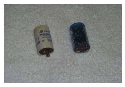
Lamp starters. On the left is a conventional analog starter and on the right is an electronic starter.
