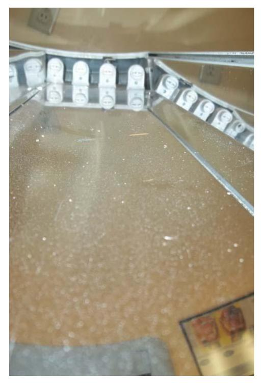
See the layer of dust on the reflector. The reflector will not perform properly with this layer of dust on it.
