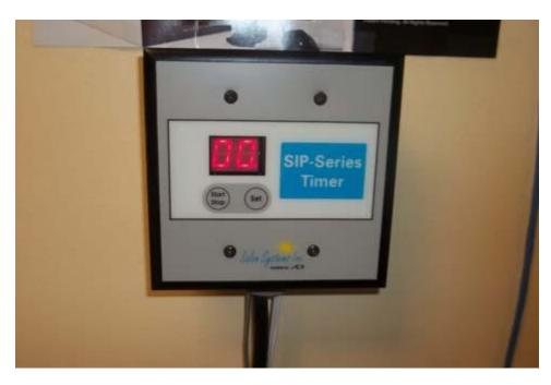
This is another example of an in-room timer. It is mounted on the wall. The client presses the start stop button before they get into the tanning unit.
