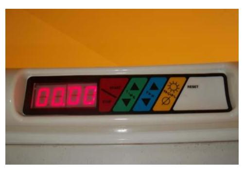
This is another example of a timer that is built into the tanning unit. In this example the client will press the red start button to start the bed or the red stop button to stop the bed.
